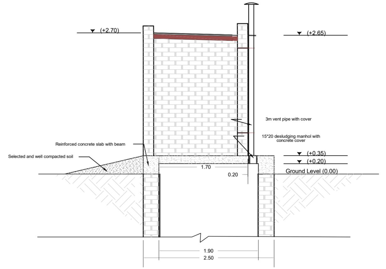
Typical section of super structure detail at (A-A)
