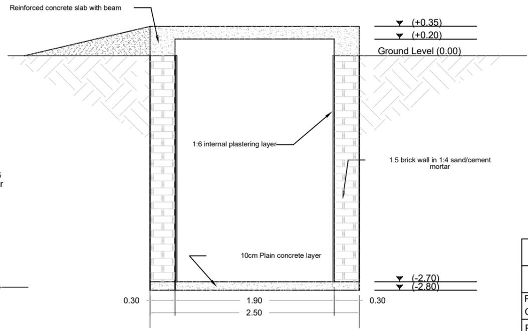
Typical section of sub-surface structure detail at (A-A)
