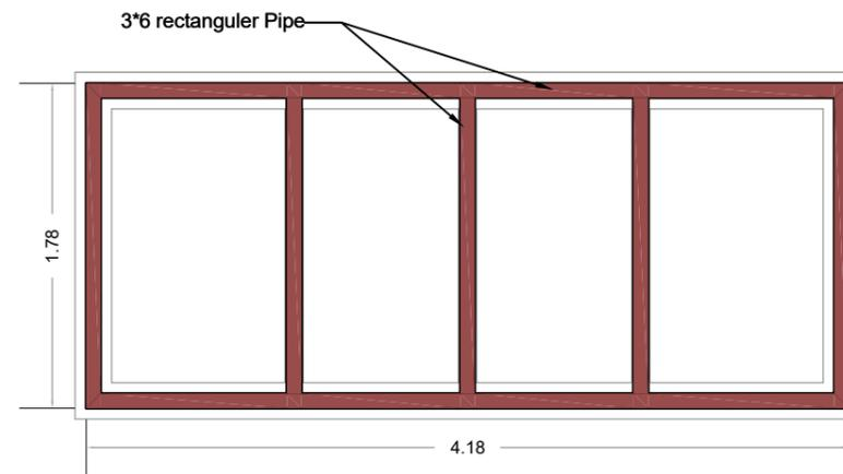
**Roof frame detail plan**
